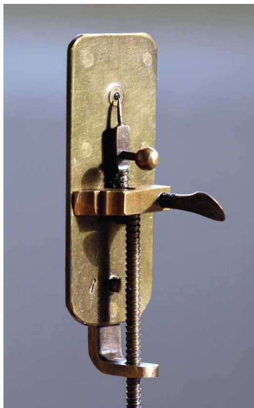
Obr. 6.2 Replika Leeuwenhoekova jednoduchého mikroskopu (By Jeroen Rouwkema, CC BY-SA 3.0, https://commons.wikimedia.org/w/index.php?curid=3657142 )
